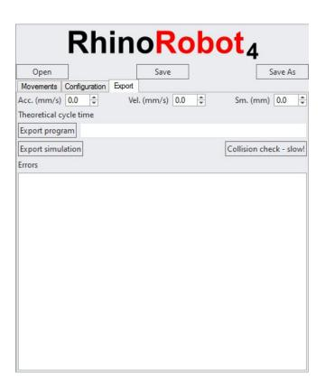
Acc: field to set the acceleration (mm/s) Vel: field to set the velocity (mm/s) Sm: field to set the smoothing (mm/s)
