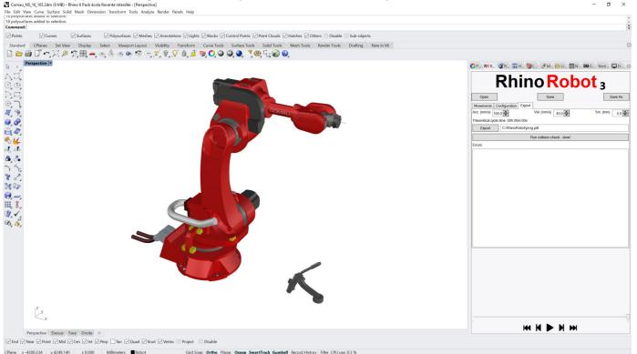
Make sure the robot is at his default angle by clicking on the reset position in the RhinoRobot panel, then place the tool on the robot flange using the Rhino "orient" command.
