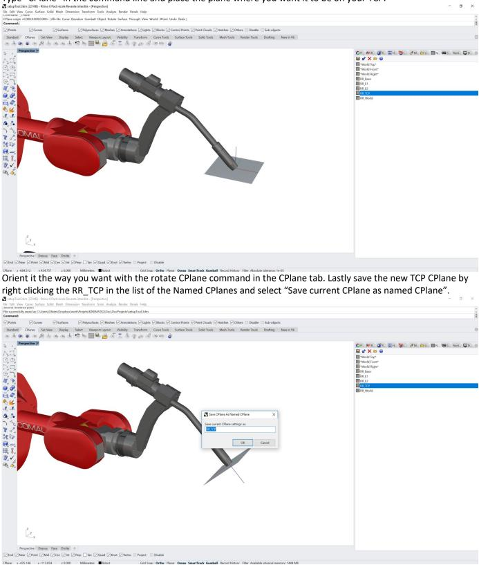
Save the project, the tool is now attached and moves as you move the robot.
