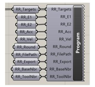
Its INPUT parameters are primarily the list of frames given by the 'Targets cluster called 'RR\_Targets' and a path for the file export. It contains the post processor specific to your robot or robot brand. To enter a cluster, just double click on its name.
