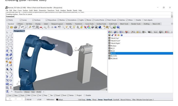
All the frames of the kinematic are calculated by reference to the robot flange, so you have to set up the curves, mesh or points in place on the tool with the robot in his default position.
