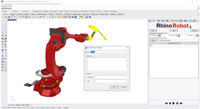
Once it is in place, select the tool geometries and type "block" in the command line, type 0 and press Enter to set (Rhino World 0) as the base point and name your block "RR\_Tool", replacing the default existing block.
