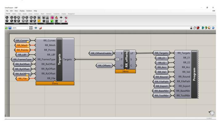
The first one, called 'Targets, is where and how the targets are constructed.
